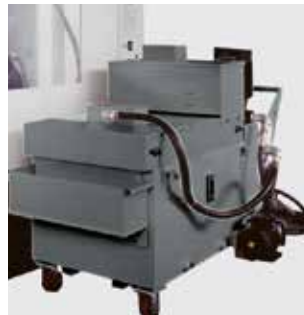
Belt filter unit on cooling water tank
